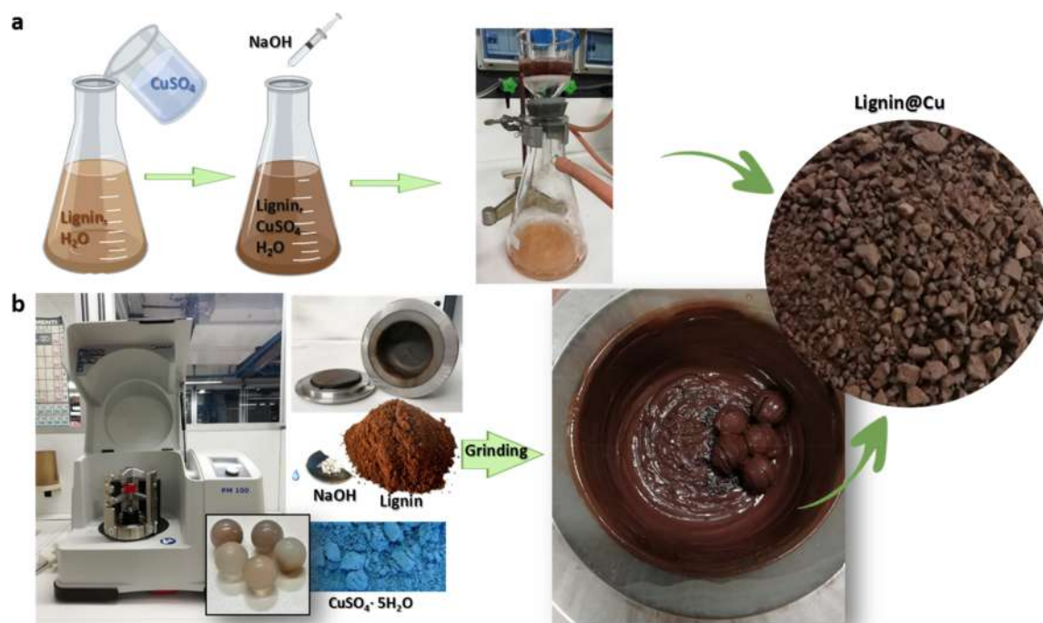
Figure 1. Comparison between the two synthetic pathways followed to obtain the hybrid material lignin@Cu: (a) wet procedure, (b) mechanochemistry.
